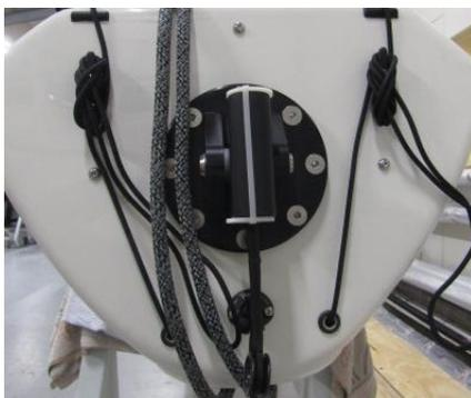
There is mounted an ANTAL padeye below the Neck bracket where the Outhaul line needs to be connected to.
