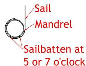
The curvature of the track fitted against lower part of the mast, helps to flatten, and correctly depower the mainsail when sailing reefed.
