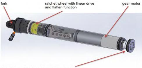
drive flange with rubber clutch turning the mandrel
