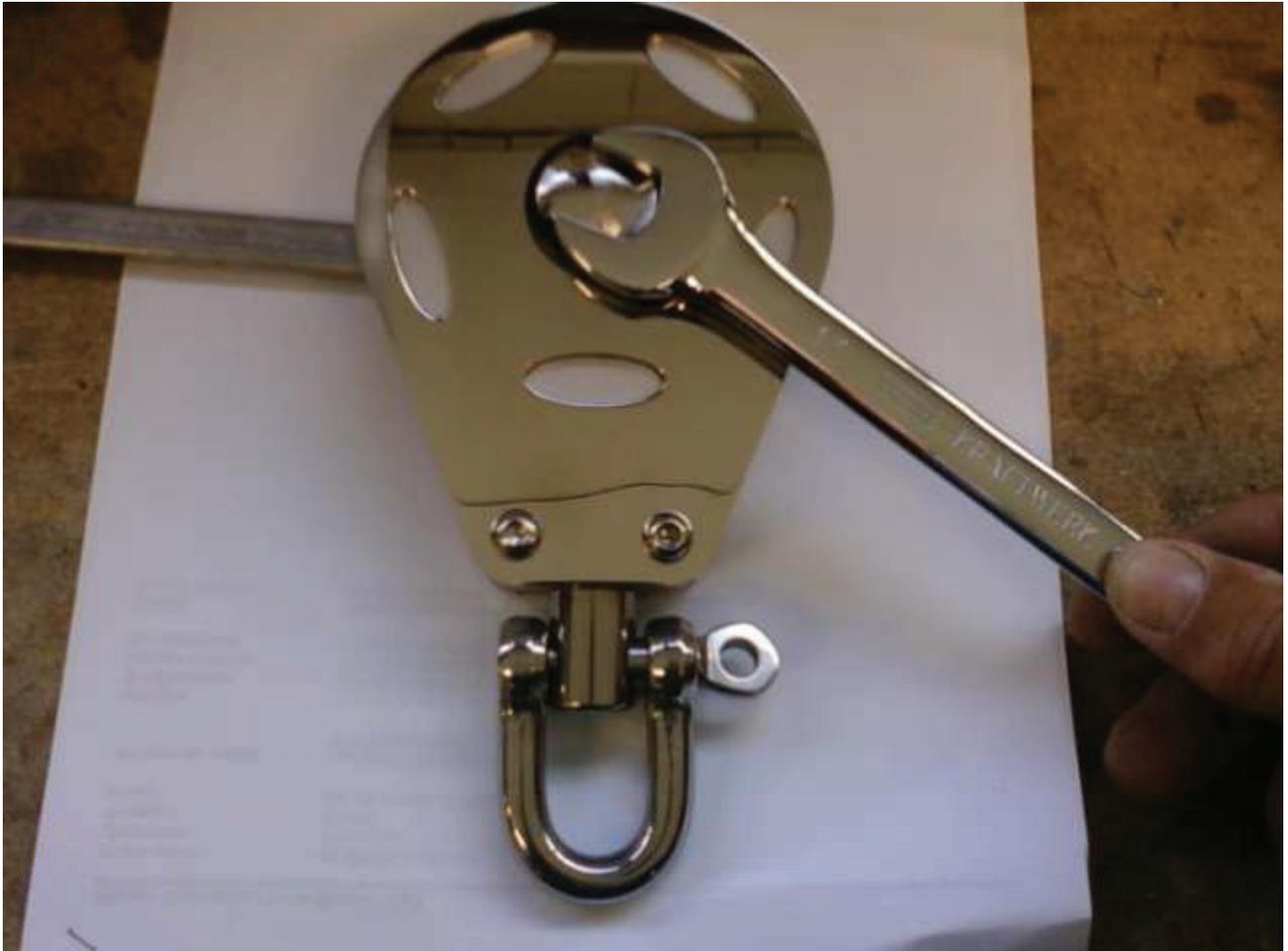
The Furlerboom main halyard control block is not a must but a help to keep the luff tight when furling.
