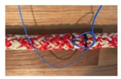
Secure the middle of the splice with some stitches. I am using regular 1mm waxed polyester whipping line. I like to finish it by making a simple" half knot", burying the ends and then cutting them.
