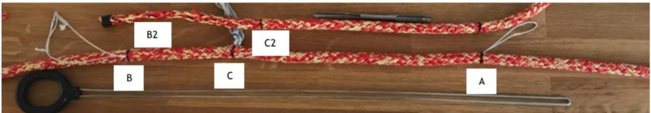
Now take the end of the loose cover (B2) and pull it in from point A and out at point B. It will be a bit difficult at the last bit, between C and B, because the core is taking up space. I recommend using a piece of 1mm Dyneema core. In the picture above, I have pulled in the 1mm Dyneema using a D-Splicer needle.
