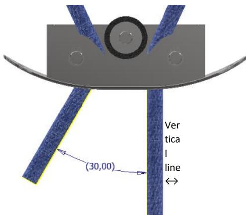
The reason why you should not pass the 30 degrees is that the furling line might tough the housing plate and because of the friction might damage the furling line over a longer period of time.
