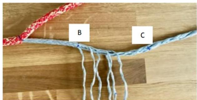
Thin out the core at point B. (The core will eventually be cut at C and thinned out all the way there. At this point I recommend taking out only 5 or 6 strands to facilitate Step 4, while keeping the structure of the braid.)
