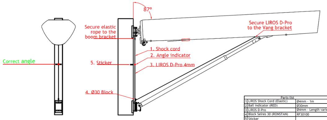
The angle indicator system consists of the following:
