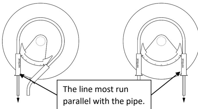
It is very important to keep tension on the line when furling! If not, you may find that a kink or knot will appear and damage the boom. We recommend to always have the line going through the stopper. This will greatly reduce the chances of causing damage to the boom and remove any unwanted kinks or knots.
