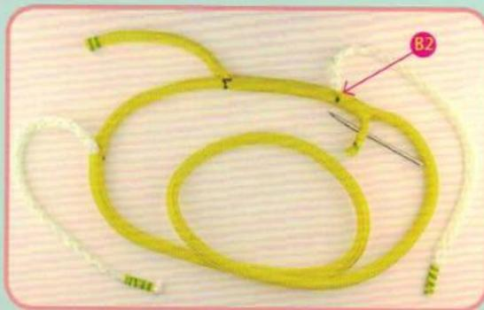
At point B2, secure the cover in place with a fid.
