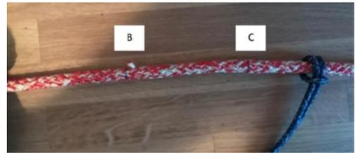
The finished splice should now have a uniform diameter throughout the whole length of the splice. If it is a little bit thicker between B and C, its usually a good thing, and it will get evened out when the furling line is used.
