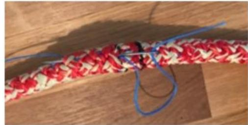
Step 6: Cut & taper the core and cover
