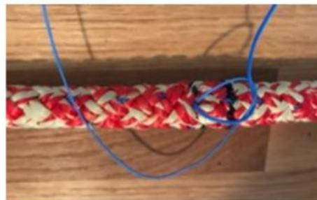
Secure the middle of the splice with some stitches. I am using regular 1mm waxed polyester whipping line. I like to finish it by making a simple "half knot", burying the ends and then cutting them. **We recommend turning the rope 90 degrees and repeat the operation.**
