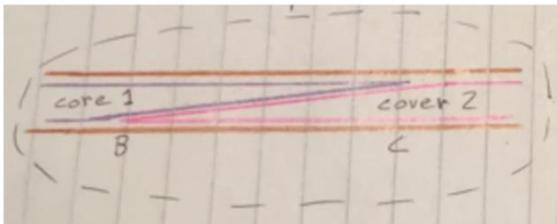
Here is a drawing that shows the basic idea of what the splice should look like. The most important part is to get a nice overlap between the core and the cover (between B and C).
