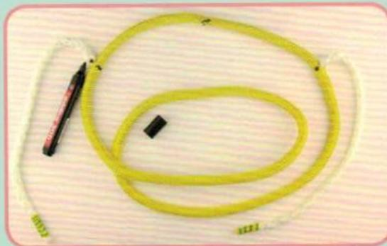
Mark the points at which the core emerges from the cover on both sides.
